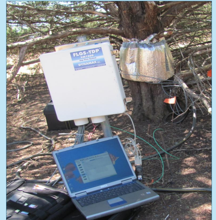
Eastern Redcedar Transpiration by Sap Flow using Thermal Dissipation Probes
