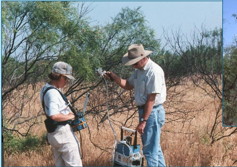
Mesquite leaf transpiration and photosynthesis using Licor leaf chamber devices
