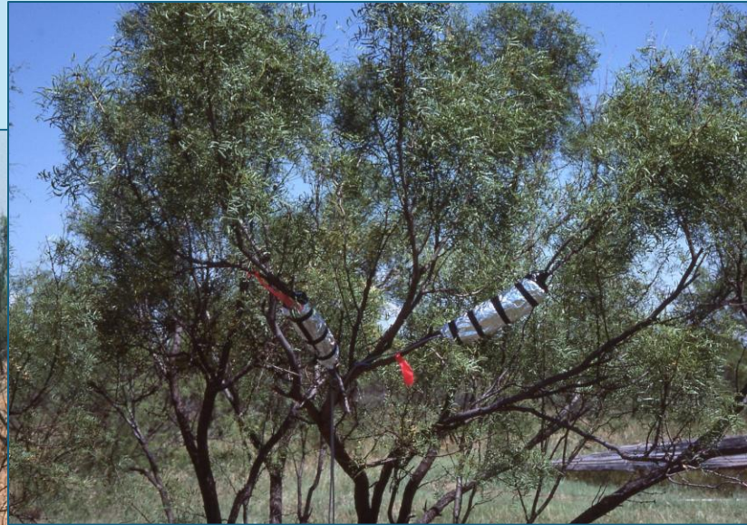
Mesquite Transpiration by Sap Flow using Dynamax SGB Gauges
